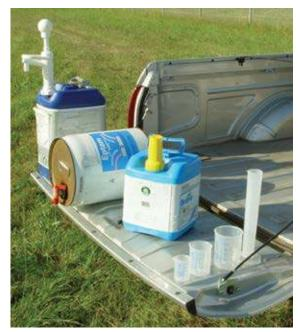
Top and below: There are various designs of taps, pumps and spouts that can be fitted to pesticide containers to reduce splash and spill risks when handling them.
