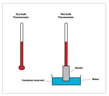
The difference between the temperatures shown by a dry bulb and a wet bulb thermometer indicate how much the temperature inside the house can potentially be reduced by evaporative cooling.
