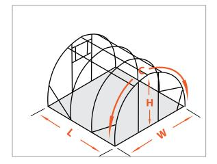
For a straight walled curved roof greenhouse, you need to measure the height of the curved section (H), the width (W), the length (L) and the length of the curved frame (C). You also need the height of the vertical section of the side (S).
