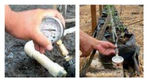
Monitoring pressure at the beginning of a lateral and at the end of a lateral.
