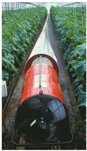
Ducted gas heating with portable gas units is not ideal but is the first step to providing effective temperature management.
