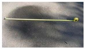
Step 2: Using water, on a dry surface, measure in metres the width of the spray pattern of the nozzle.
