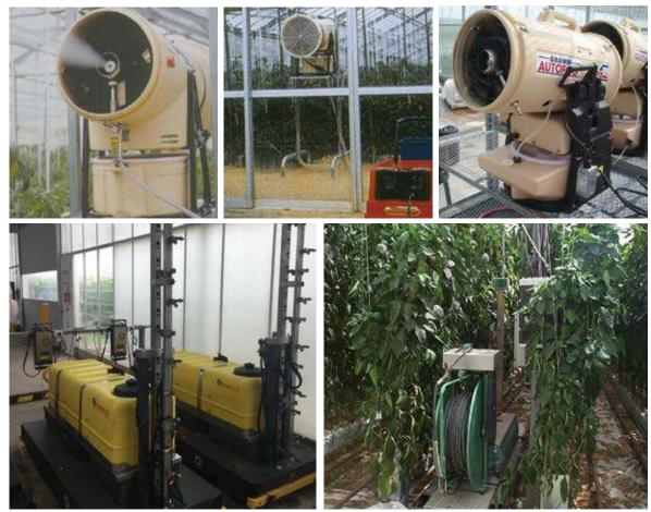
Above: Different makes of remote or unmanned sprayers are available that reduce exposure risks when spraying pesticides in greenhouses.
