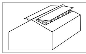
Twin roof vents, preferably with insect proof mesh, offer excellent Single roof vents on enclosed higher tech greenhouse. venting capacity under most conditions.
