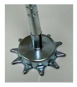
7. For proper operation, the wheel ferrules must grip the shaft firmly without slippage. Also, a slight gap between the wheel ferrules and the body of the seeder must be present so the wheels and axle will turn freely without friction.
