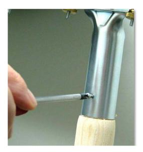
3. Using a #1 Phillips screwdriver, secure the seeder body onto the handle with the #4 x  $\frac{1}{2}$ -inch wood screw provided.
