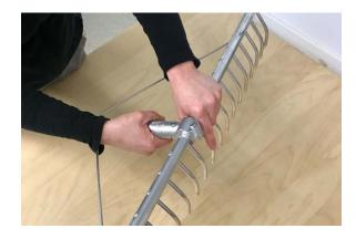
**4.** Fasten the support arms using a Phillips head screwdriver.
