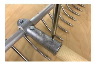
2. Loosen the bolts on the top of the rake head so you will be able to adjust it to your desired angle. \*Exact wrench size is recommended to avoid stripping the bolts.
